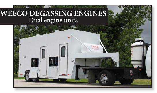
3 million Btu/Hr. Combustion Capacity 400 cubic feet per minute per engine Electronic air-fuel control Filtered tank vapor extraction blower Filtered air injection blower Propane or other fuel option NOx and HC/CO catalytic converters Sound buffering enclosure VOC detectors and exhaust analyzers Flame arrestors and detonation arrestors KO drum and flow sensors Auto/Safety shutdown system
