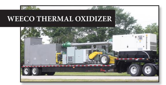
15 million Btn/Hr. Combustor on VFD Controls 5,000 cubic feet per minute Automatic fuel-air ratio control Diesel engine based electric generator (145 Kw) Filtered air injection blower Filtered tank vapor extraction blower Propane or other fuel option
